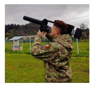
The Silenta 6001 UAS Counter-UAS System is a non-kinetic, portable, self-contained defensive equipment designed to neutralize unmanned aerial vehicles (UAVs) by disrupting the primary control and navigation signals used by commercial UAS and S-UAS systems.
